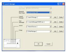
Launch Manager allows you to set the four launch keys located above the keyboard. "Launch keys" on page 8 for the location of the launch keys.
